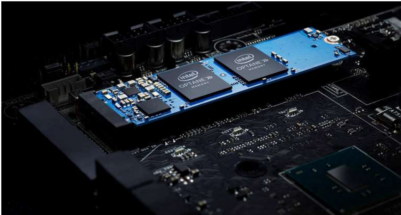
Figure: Optane memory installed on a mainboard [229]
