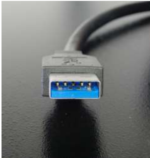
Figure: Front view of a Standard-A USB 3.0 connector, showing its front row of four pins for the USB 1.x/2.0 backward compatibility, and a second row of five pins for the new USB 3.0 connectivity (above). The plastic insert is in the USB 3.0 standard blue color.
