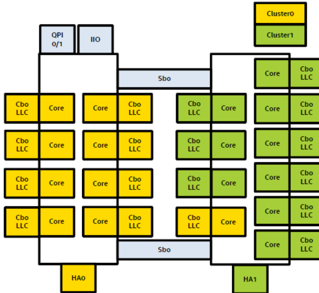
Figure: Partitioning 18 cores into 2x 9 cores for the COD mode in a Haswell-EP processor [134]
