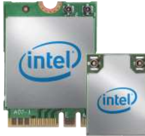
Figure: CRF modules implemented on an M2 card or as a compact bridge chip [164]
